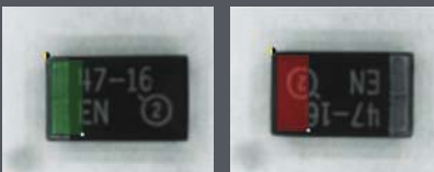
Capacitor oriented correctly
