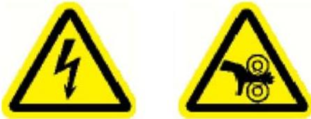
**Disconnect the power from the machine before you perform the following procedures or you may be injured by the moving drive belts and pulleys, or receive an electric shock.**
