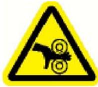
Disconnect the power from the machine before you perform the following procedures or you may be injured by the moving drive belts and pulleys, or receive an electric shock.
