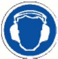
This symbol indicates a high noise level is present. Ear protection must be worn to avoid hearing loss.
