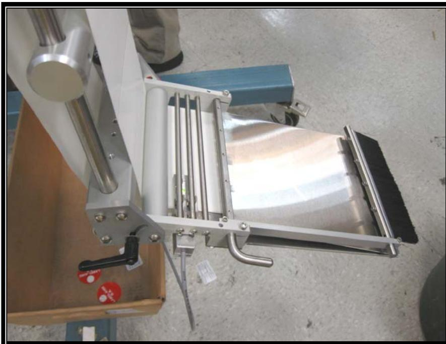
Figure 19 LABEL SENSOR & PEEL TIP ASY
