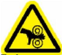
The potential for finger pinch exists between the drive and pinch rollers. Keep hands clear of the drive and pinch rollers whenever the machine is ONLINE.
