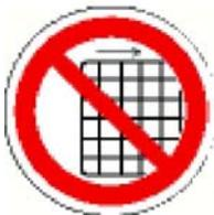
This symbol indicates that the machine should not be operated unless the covers/guards are in place.
