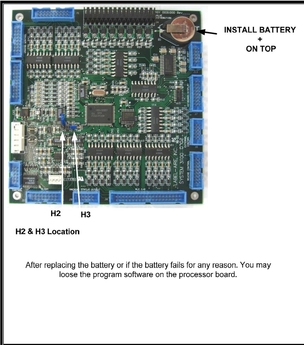
Figure 35 Control Board H2 & H3 location
