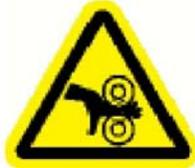
Disconnect the power from the machine before you perform the following procedures or you may be injured by the moving drive belts and pulleys, or receive an electric shock.
